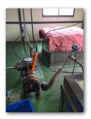
3" ANSI 2500- EDS valves were N2 tested after immersion in cold box at -46C to validate the performance of the EDS seat design with the Delta seat / Viton seat carrier O-rings.
