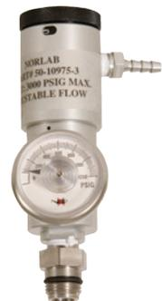
The 8000 Series regulators are used for calibration of instruments that draw the gas mixture with an internal pump. Constructed of stainless steel and aluminum, they are compatible with reactive and non-reactive gas mixtures. They supply flows of 0.1 LPM to 3.0 LPM, and are suitable for use with high pressure refillable cylinders as well as non-refillables.
