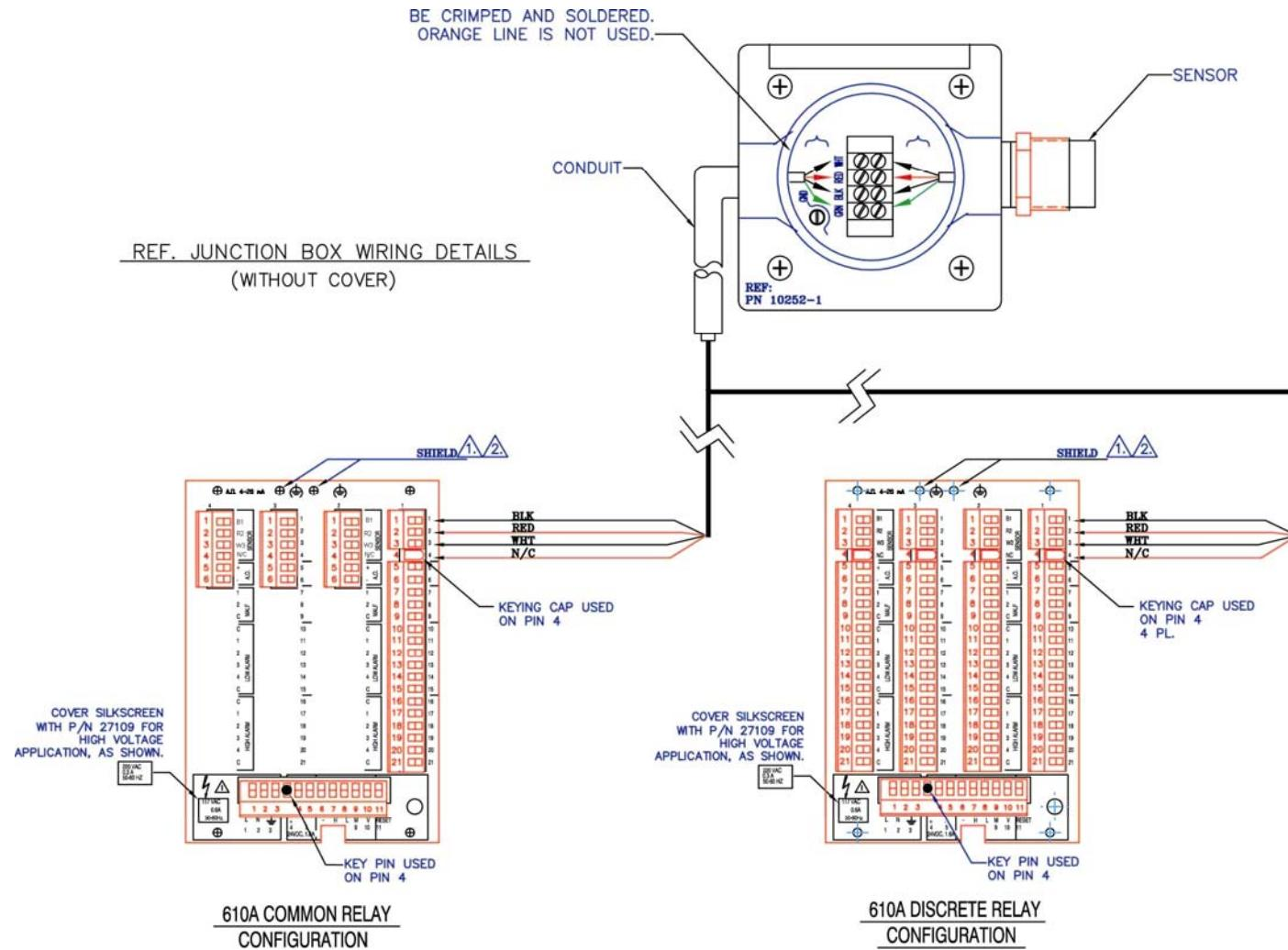
**Figure 3: Outline Drawing & Rear Terminal Connections (REF: 20659)**
