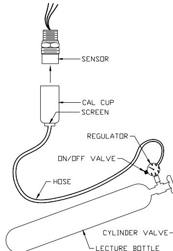
**Figure 9: Portable Purge Calibrator**
