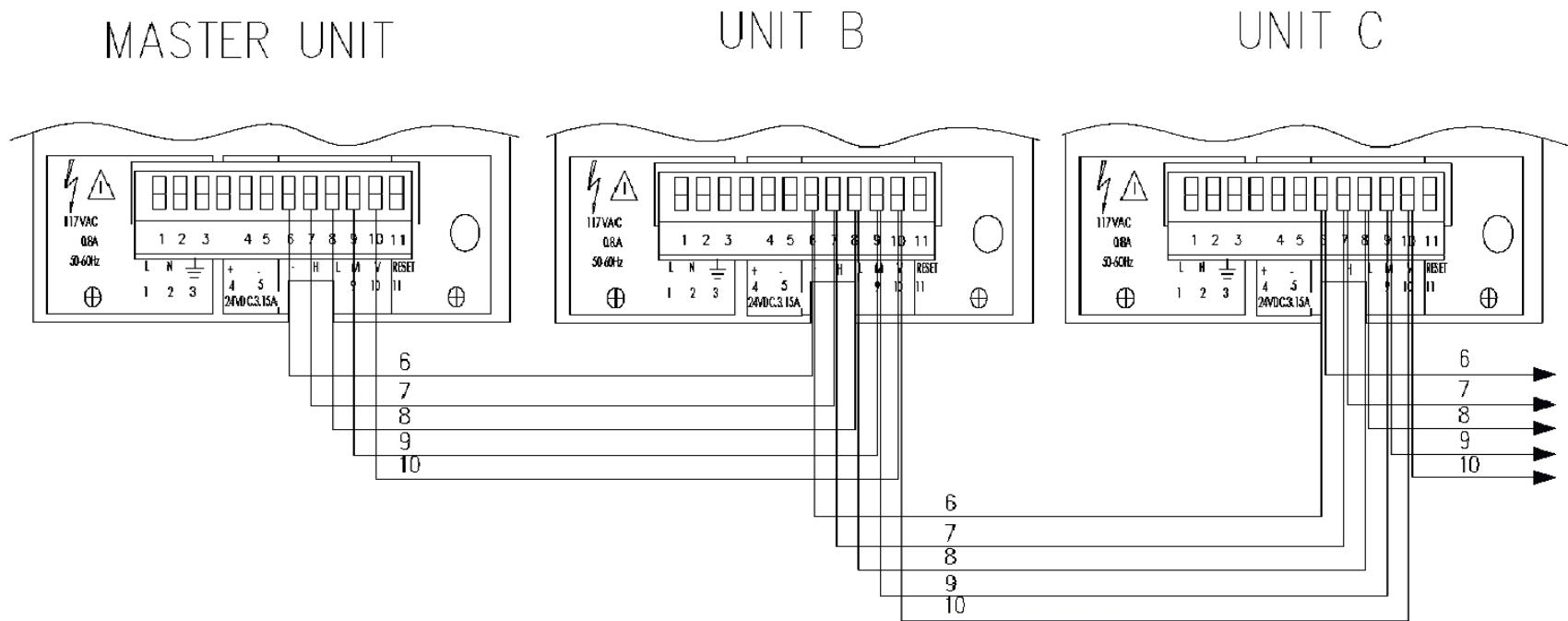
**Figure 11: Interconnection Drawing Zone Control Model 610A Controller**
