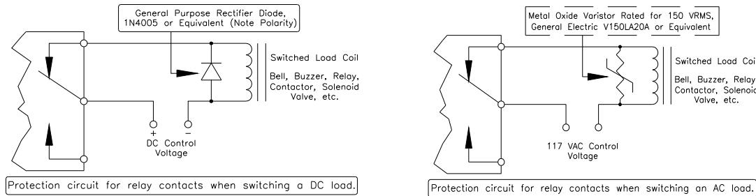
**Figure 7: Protection Circuit for Relay Contacts**
