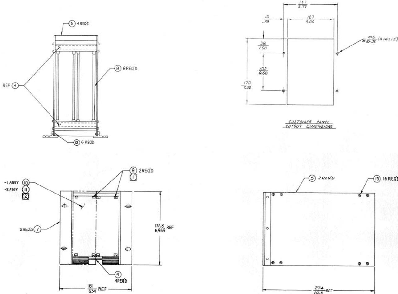
**Figure 10: Panel Assembly, Panel Mount –98, Ref: 10199C**
