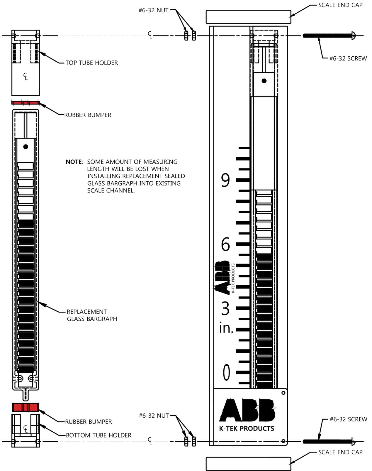
**Figure 5.7-4 KM26 Bargraph Replacement Glass Installation Procedure**
