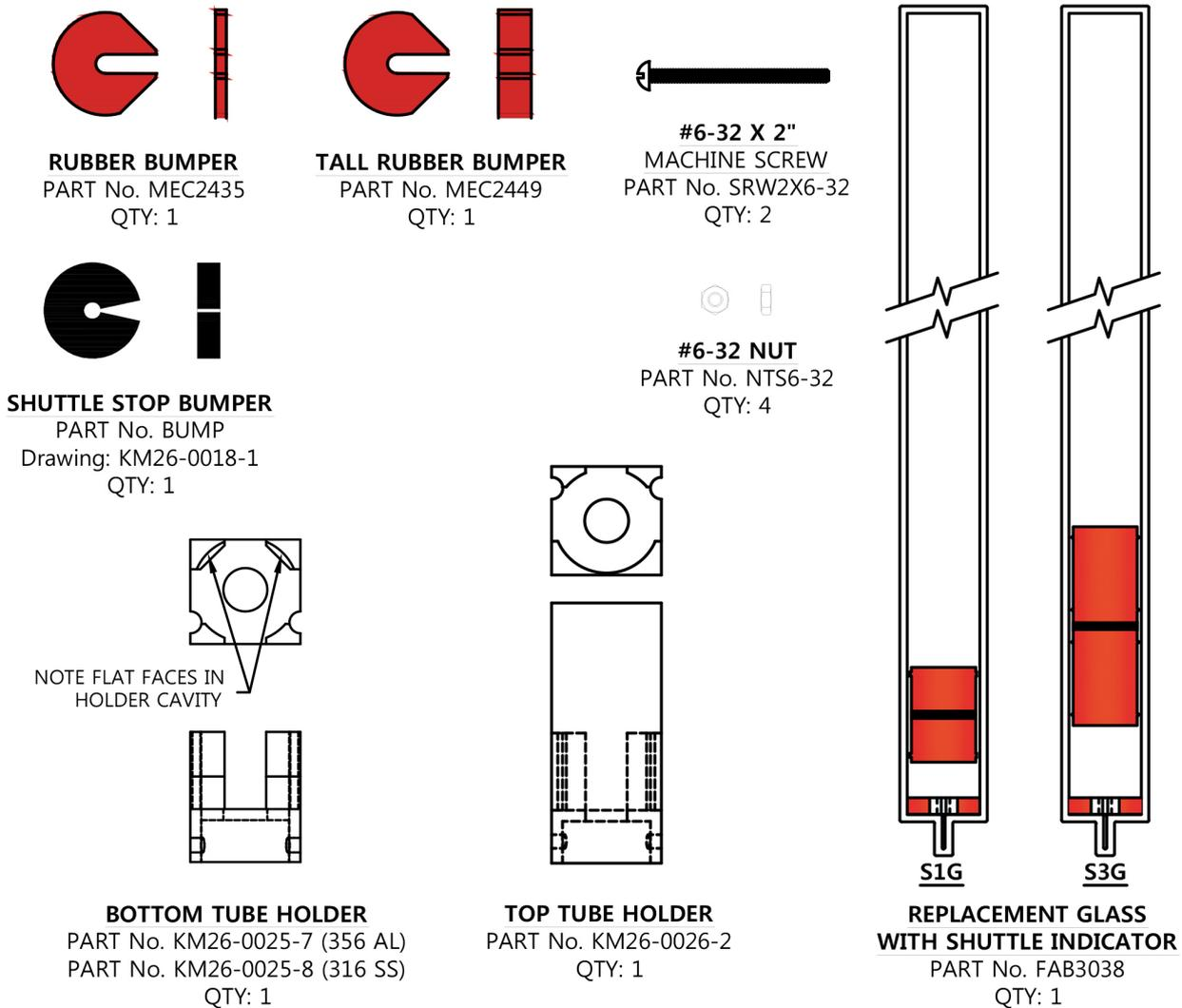
Figure 5.7-3 KM26 Bargraph Replacement Glass Installation Procedure
