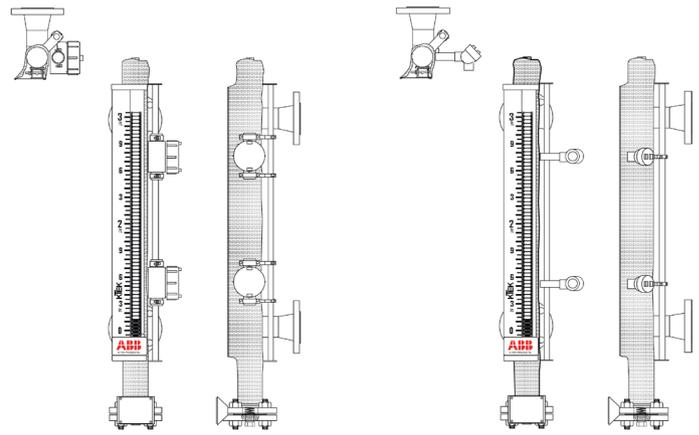
**Figure 3.8-1 MLG with Switches**
