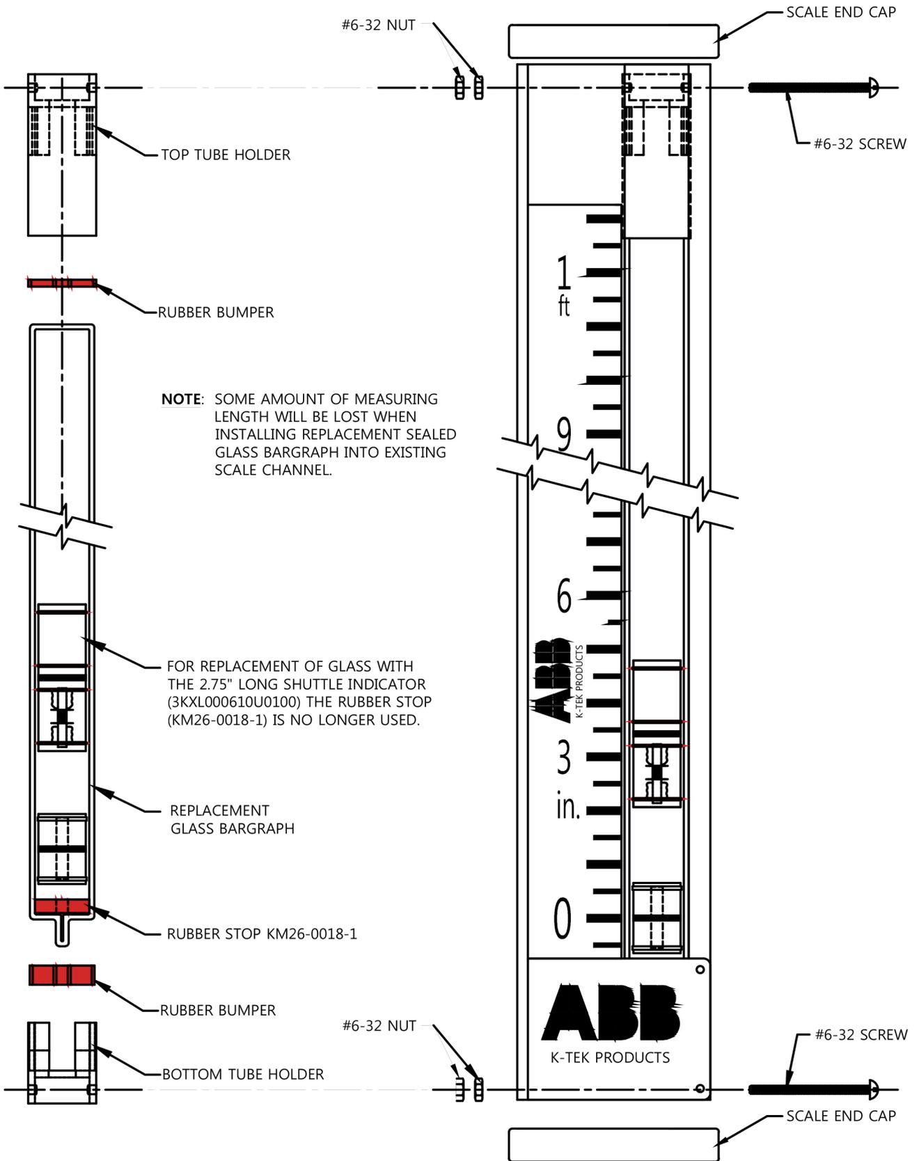
**Figure 5.7-2 KM26 Shuttle Replacement Glass Installation Procedure**
