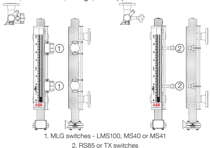
Figure 3.6-1 KM26 with Level Switches
