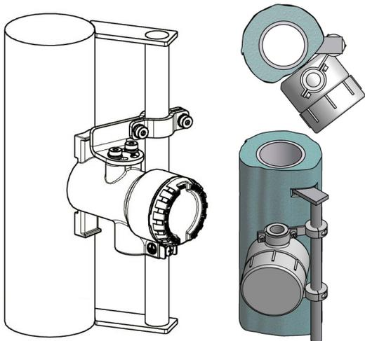
Figure 3.7-2 MLG Switch with Insulation Jacket with Rod Mounting
