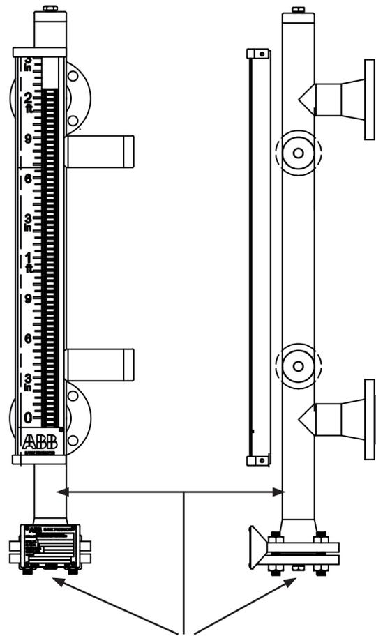
Possible grounding locations with a pipe clamp, pipe strap or ring terminal on flange stud
