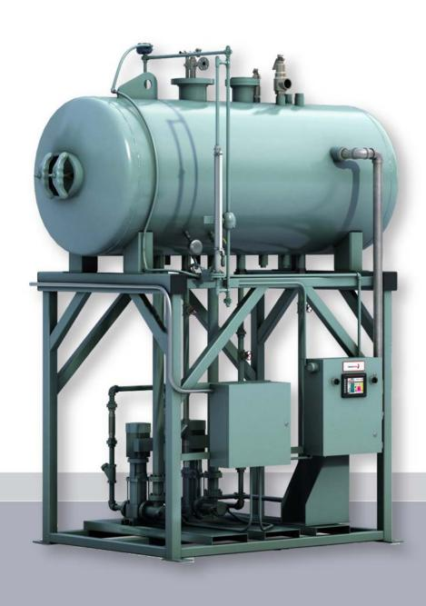
The Cleaver-Brooks designed deaerator assures high purity effluent by removing oxygen and other dissolved gases in boiler feed. Thus, it is the answer to long- lasting boiler equipment for industrial and commercial boiler users. Built of corrosion-resistant alloys for lifetime service, the deaerator employs those basic principles of gas removal proven most effective and economical to every boiler owner. Contact your local Cleaver-Brooks authorized representative for component sizing information.
