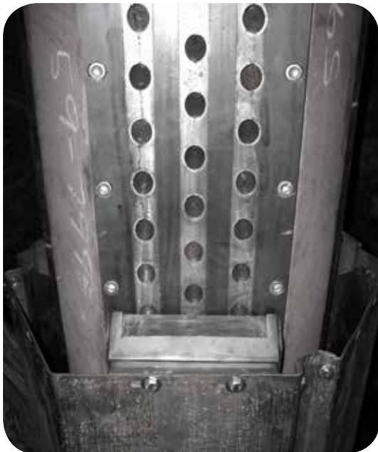
**Control Sleeve Intercepts Jets to Modulate Capacity**
