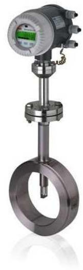
Figure 5. Thermal mass flowmeters introduce heat into the flow and measure its dissipation. They measure at a point within the gas stream.
