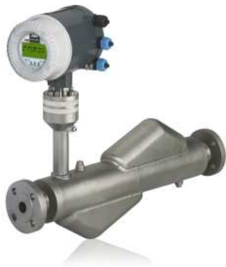
Figure 4. Coriolis flow tubes come in a variety of shapes, depending on the manufacturer. Above is the S-shape of ABB's Coriolis flowmeter.
