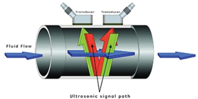
accuracy is limited by how precisely the time is measured. There is a practical limit both technologically and commercially, on what level of resolution in time measurement can be achieved. Another way to improve precision with the same resolution in time measurement, is to take more measurements. This is done by adding a second path, another set of sensors, to make another set of time measurements with the same resolution.
